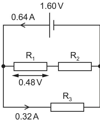
The cell has electromotive force (e.m.f.)  $1.60\text{ V}$  and negligible internal resistance. The current in the cell is  $0.64\text{ A}$ .
